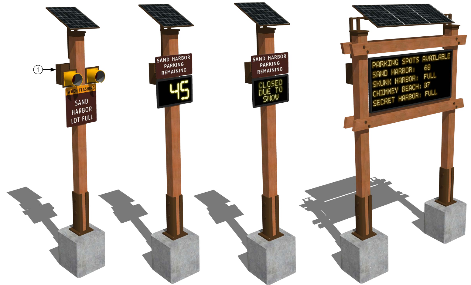
Example use of a standard sign post with future electronic sign options, from basic flashers to advanced digital displays
