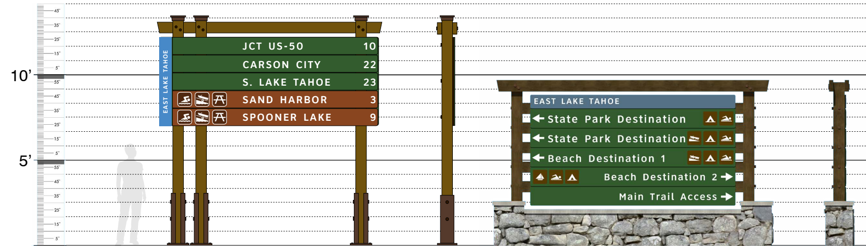
Sign Type A Vehicular Pole-Mounted Directional
